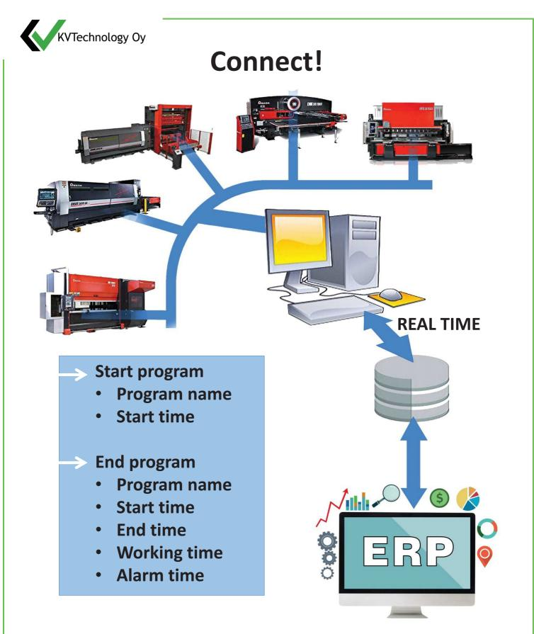
With **Connect!** it is possible to connect Amada production machines to any ERP- or MES- system
